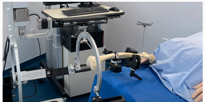
Seen here under development, Robossis will be the first navigation system to robotically situate femur bones for surgical repair of fractures.
