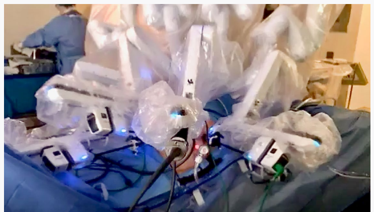
A da Vinci robotic laparoscopy system is mounted and docked to begin a sigmoidectomy for diverticulitis.
